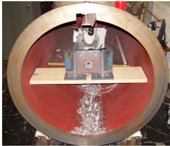
Figure 8. Open catch tank showing sabot catcher in front with sample mounted in back.
