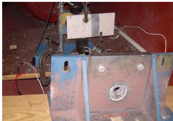
Figure 9. Picture of the metal sabot “stripper” with a sample plate and two mounted photodiode detectors facing sample.
