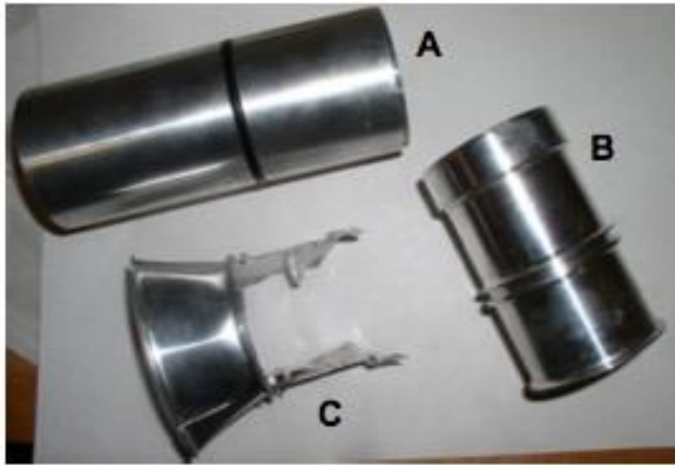
Figure 6. Pictures of: A) 1.2 kg sabot, B) 90 g sabot, and C) 90 g sabot after it was shot through the catch “stripper.”
