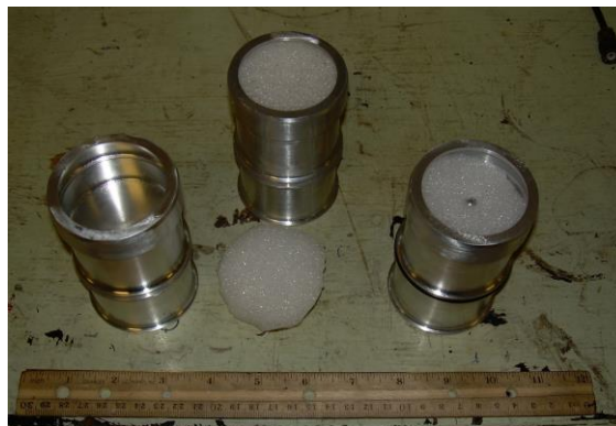
Figure 7. Picture showing (from left): blank sabot, sabot with added foam insert, and sabot with foam insert and loaded projectile.
