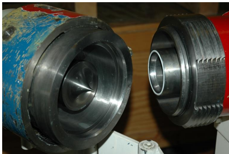
Figure 5. Picture of the open gun breech chamber showing the firing pin on the left and the sabot loaded on the right.
