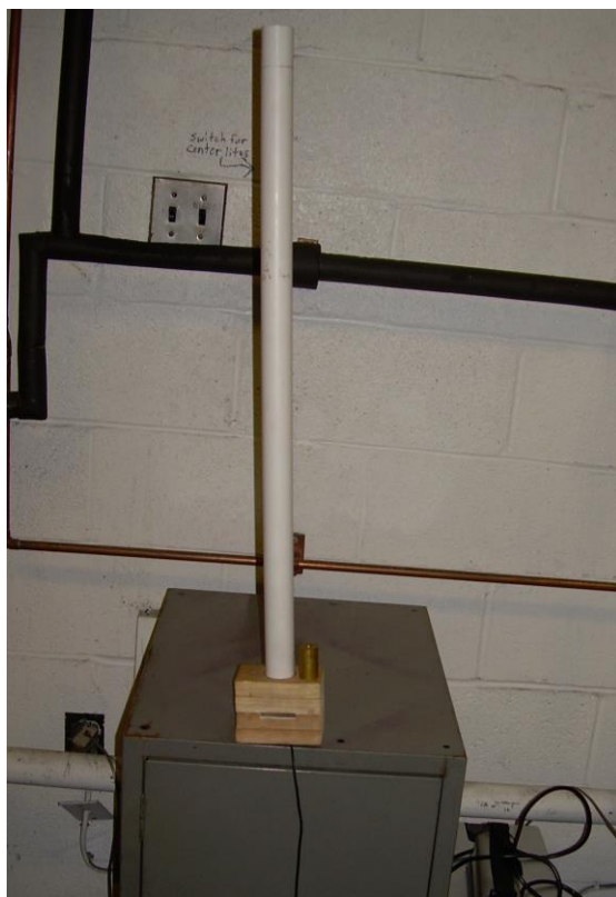
Figure 1. Picture of the drop tower used for low speed TL testing.
