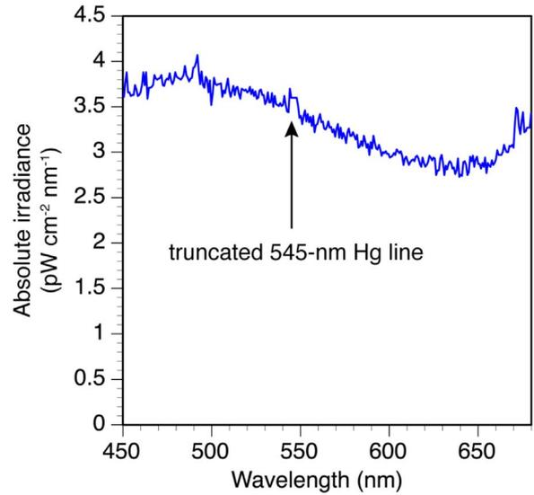
Fig. 4. Measured absolute spectral irradiance at fiber cable end from glass fluorescence (average of two trials). Incident 253-nm UV radiation was  $5.35 \mu\text{W cm}^{-2}$ .
